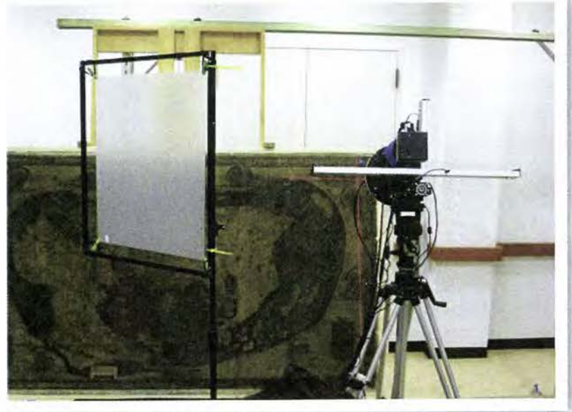
Scientists are now using a technique which involves capturing multiple images of the map at specific frequencies of light, including ultraviolet and infrared. The images are digitally combined and processed in a way that uncovers information otherwise hidden to the naked eye
