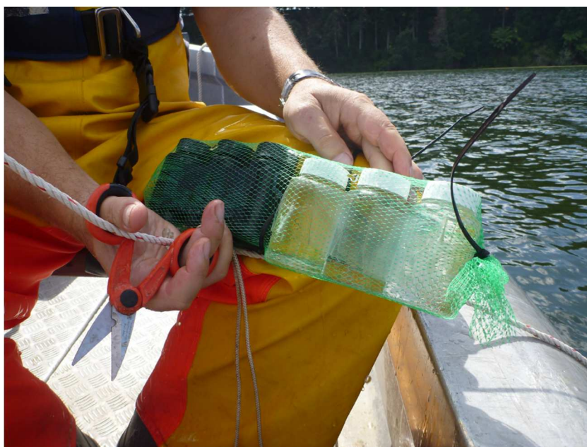
Figure 4: PPR bottles assembled in a net bag attached to an incubation line ready for deployment. The dark control bottles were painted black and covered with black tape.
