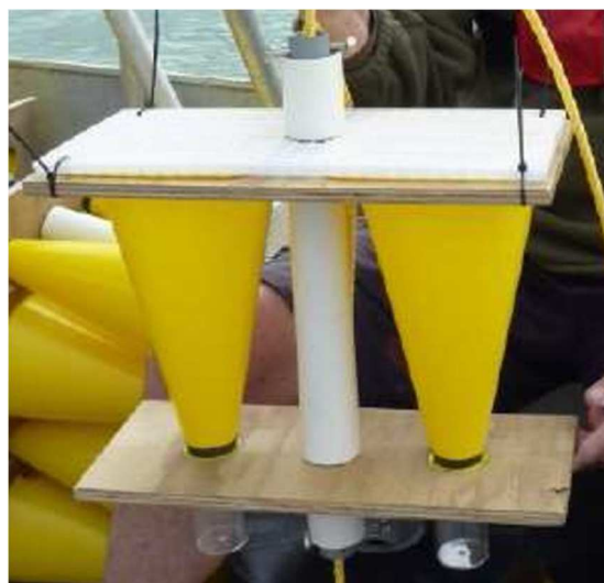
Figure 5: Dual collector sediment traps. Upper cone opening is 150 mm diameter covered with a 10-mm square grid plate. The sediment is collected in 60 ml screw-cap jars.
