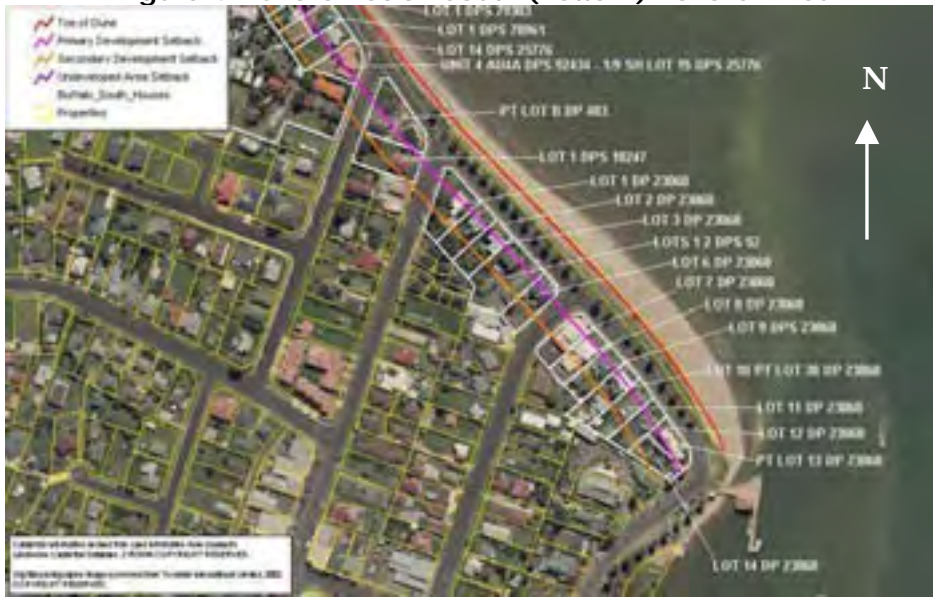
Figure 4: Buffalo Beach South (Bottom) Hazard Lines
