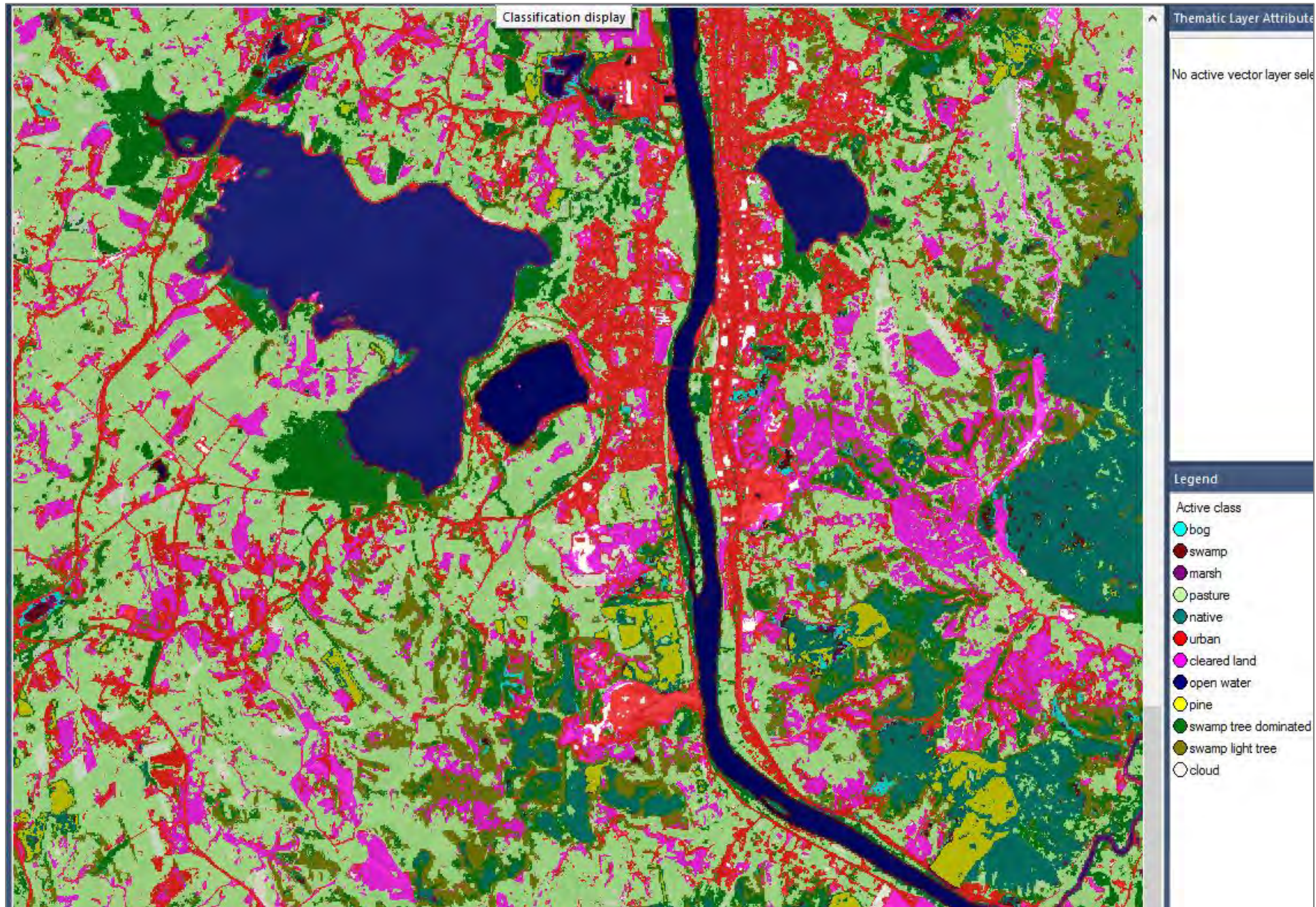
Figure 5c. The results of object oriented classification of the Huntly area, without polygon boundaries.
